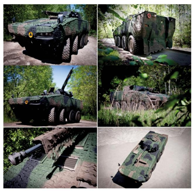
Mobile Camouflage provides multispectral mobile Protection VIS, NIR, TIR, RADAR.
