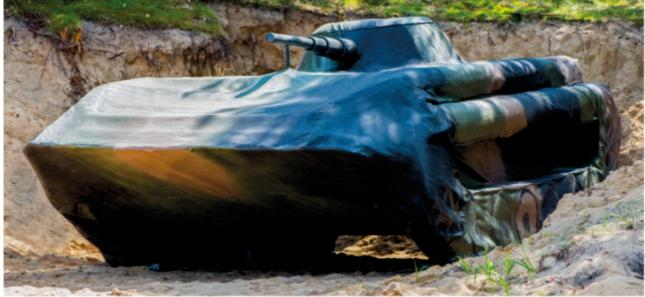
The inflatable mockup is designed to simulate individual objects or groups of equipment in mixed (mockups and real equipment) or simulated (only mockups) conditions. Inflatable mockups simulate the presence of the equipment in a wide spectrum of electromagnetic radiation used in the reconnaissance, i.e. in the visible, thermal and radiolocation range.
